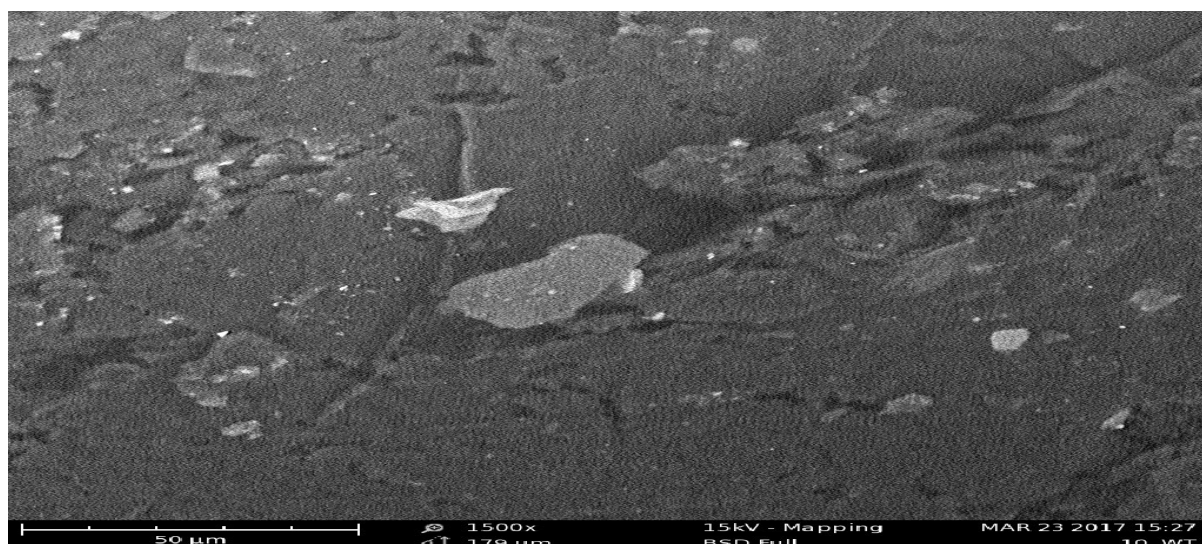
Figure 10: SEM Photography of non treated bagasse reinforced LDPEC
