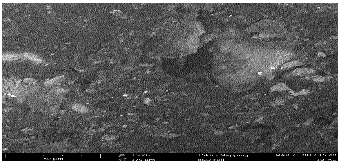
Figure 11: SEM photograph of acetylated treated LDPEC
