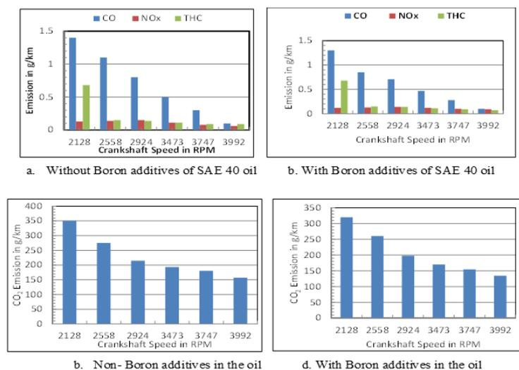
Figure 9: Effects of engine speed on fumes using CNG for SAE 40 lubricants
