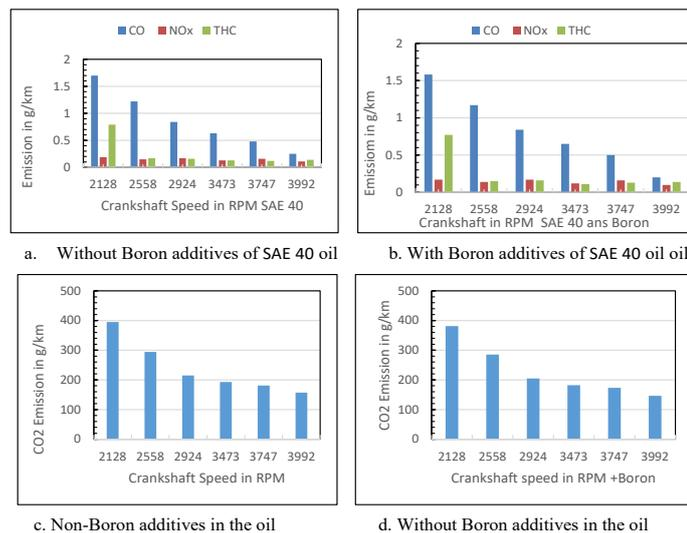
**Figure 12:** Differences in emissions with engine speed when using SAE 40 lubricating oils and gasoline
