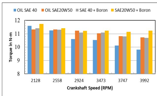
Figure 8: Variance in oil torque in relation to speed combinations using petrol as fuel
