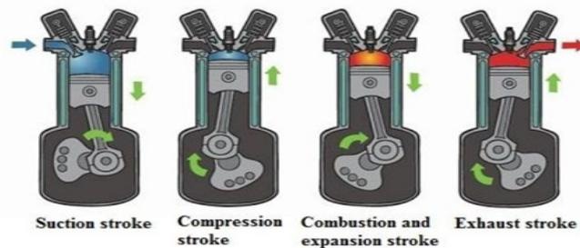
**Figure 2:** Cycle of operation of four-stroke engine (Korakianitis et al., 2021)
