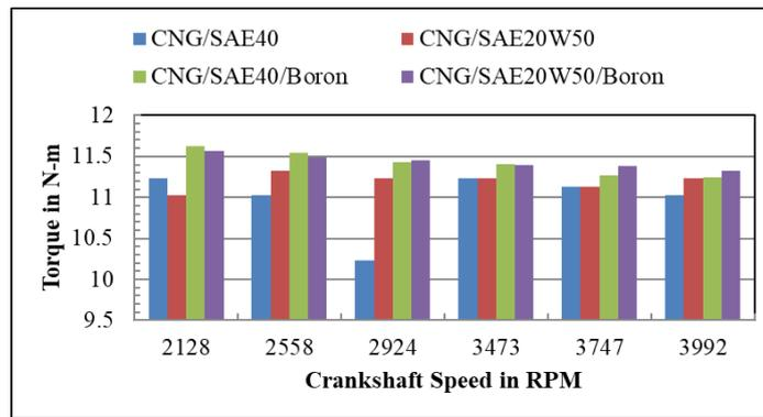
Figure 7: Torque fluctuations in relation to speed for oil mixtures utilizing CNG as fuel
