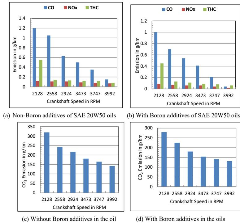
**Figure 10:** Changes in emission with engine speed using CNG for SAE 20 W50 lubricating oils
