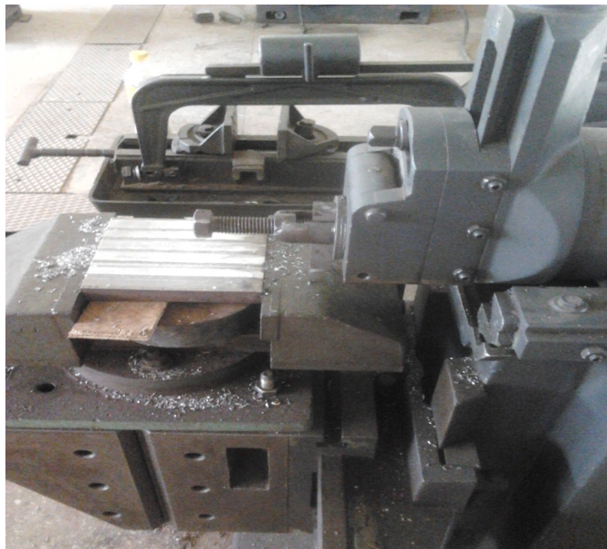
Plate.1: Machining the 12.9cm X 12.6cm X 1.9cm Mild Steel work piece
