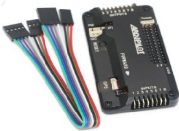
Figure 2: APM Flight Controller. Figure 3: ESCs and Propellers. Figure 4: Lithium ion Battery.
