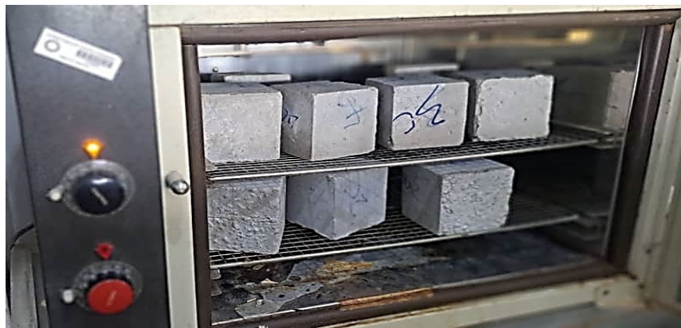
Plate I: Burning of Bioconcrete at Elevated Temperature
