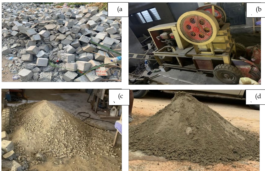
Figure 1: Recycled aggregate preparation (a) concrete cubes waste (b) mechanical crusher (c) crushed concrete waste (d) recycled fine aggregate
