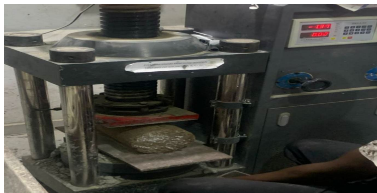
Figure 3: Split Tensile Strength Test on Concrete Paver Block
