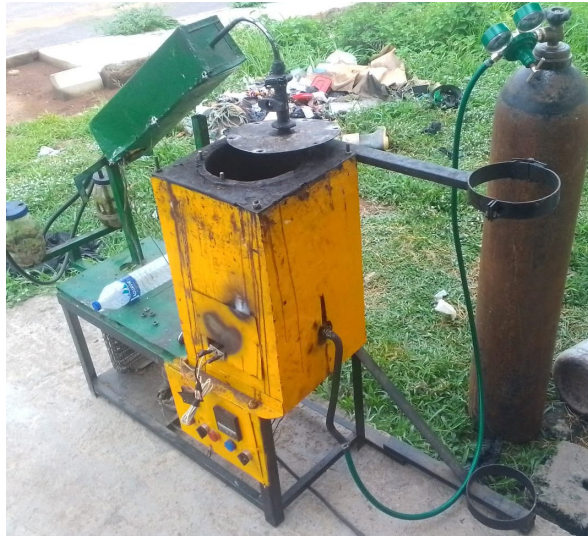
Figure 2. The pyrolysis setup used for the experiment
