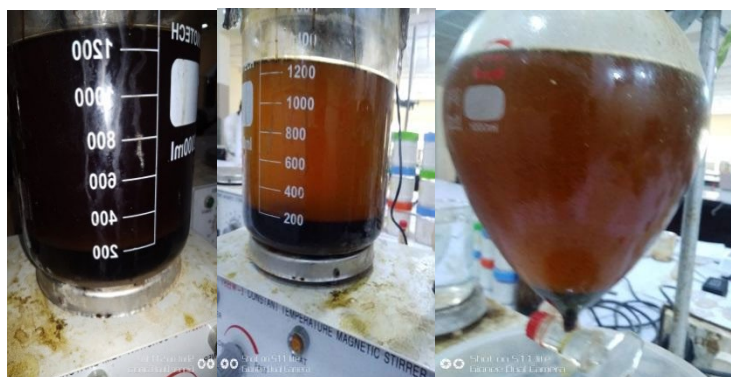
Figure 5: Pictorial representation of biodiesel separation from glycerin
