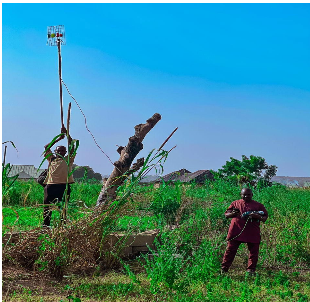
Plate 1: A photograph showing the placement of the Yagi antenna and the Spectrum Analyzer for the measurement of RF at one of the study locations
